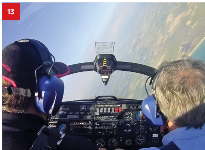
13 Back to the harder stuff, this time an accelerated stall which ends with a violent flick into an incipient spin... "and recover." It's the same technique – Push-Roll-Thrust – and it's starting to become second nature now
