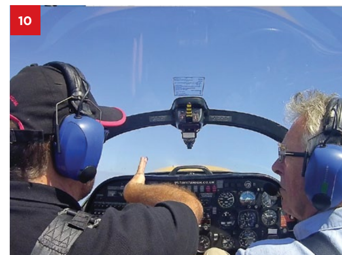
10 Up 'til now, it's been straightforward but Mark's about to put the Firefly into a sideslip as though on final approach, slow speed, high Angle of Attack so the Firefly stalls. He talks me through it before doing it...
