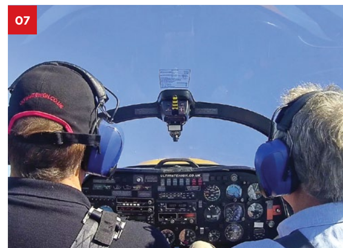
07 We carry out the same stall exercise but this time with some angle of bank, just to add another layer. It's the same recovery technique though. Push the stick centrally forward, Roll wings level, adjust Thrust
