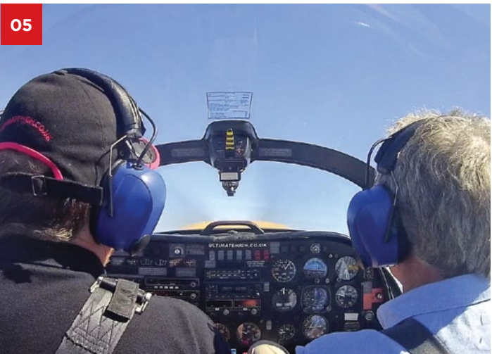
05 So now Mark is putting the aircraft into a stall with the throttle closed. Speed is decreasing (see the ASI), we're climbing slowly and there's a bit of buffet. The wing drops... "and recover." He's good at saying that
