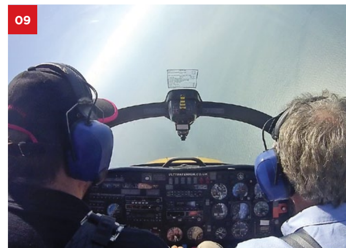
09 A spiral dive is a touch scary so the simple mantra "Push-Roll-Thrust" is the only thing going through my rapidly getting maxed out brain. Reducing power quickly is vital as is gently pulling back on the stick, not rushing it
