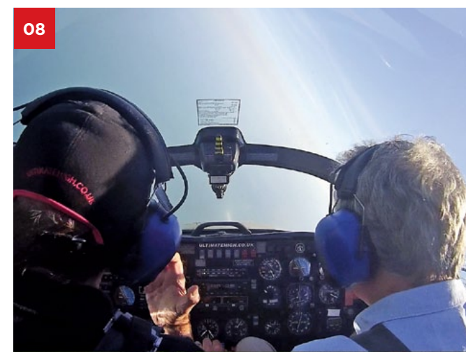
08 Moving on, this time it's a spiral dive which can be disorientating. Nose down, wings banked, speed increasing, vertical speed indicator (VSI) going off the clock... it's that blinking phrase again, "and recover"
