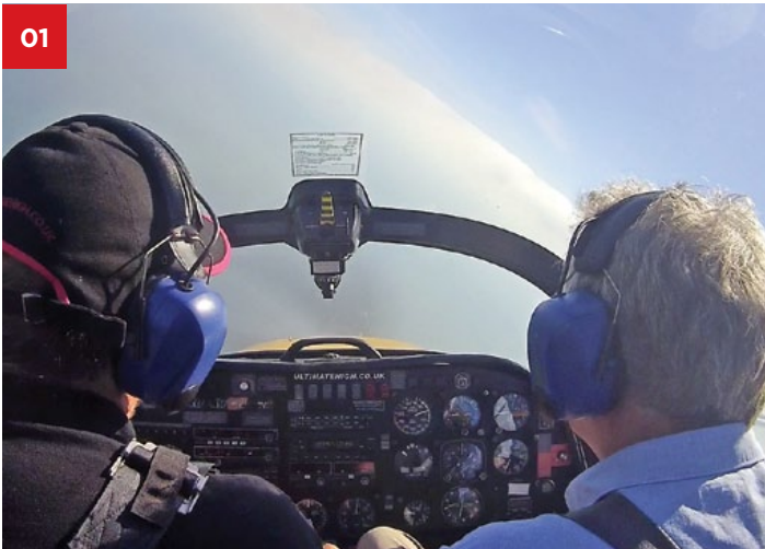
01 Upset Recovery Training with Ultimate High is in a Slingsby Firefly and starts with simple recovery from a nose low attitude with a slice of steep bank thrown in, induced by instructor Mark, in the left seat
