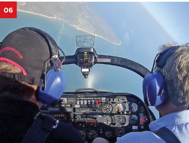
06 Getting the aircraft flying again is critical so reduce the Angle of Attack and unload the wing. Push the stick centrally forward and centre rudder pedals. As the airspeed rises, roll the wing level and adjust Thrust
